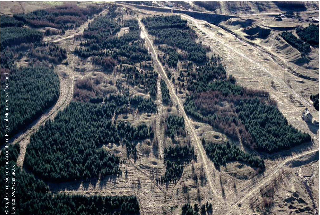
Figure 15. The site of Wilsontown Iron Works, showing a series of circular bell pits.
